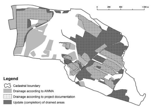
Fig. 9. Example of differences in area drainage according to the design documentation (created vector layer) and according to the AWMA data – the model locality of Žejbro, selected cadastral district of Radčice u Skutče.
