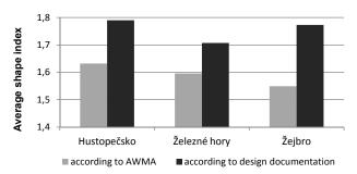
Fig. 10. Comparison of the average drained area shape index according to the AWMA records and the vector layer from design documentation in the model localities (shape irregularity increases with increasing value).
