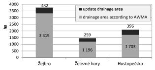
Fig. 8.The size of drained areas according to the AWMA and the addition of missing areas according to the vector layer from design documentation in the model locations.
